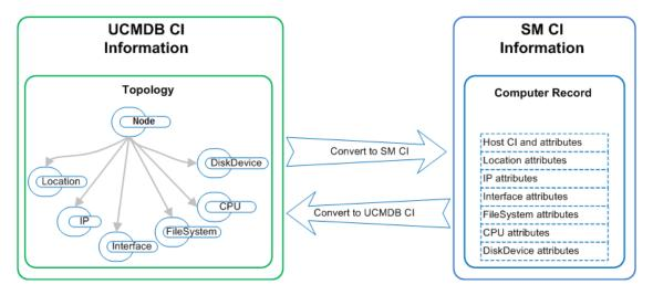
The above figure shows the correlation between the UCMDB topological model and its representation of the Computer Instance together with its parallel representation in SM. The SM computer CI contains all of the UCMDB information that is passed through the integration.
